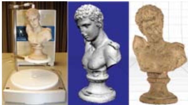
The original object is scanned in a 3-D scanner (left), turned into a cloud of points (center), and then into a surface model.
