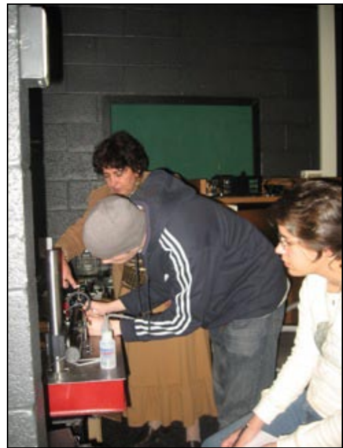
Dr. Dushkina and a student are fine tuning a laser assembly in the dark lab. Notice how the walls are painted black to minimize reflections.
