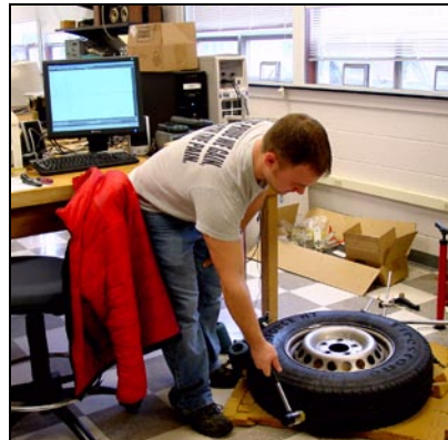
A student strikes a tire with a hammer. By analyzing the acoustic response of the tire, Dr. Dooley and the student hope to gain insight into the structural integrity of the tire.
