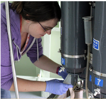
An oceanography student takes a seawater sample from a Niskin bottle sampler aboard the RV Knorr, North Atlantic Ocean, spring 2014.
