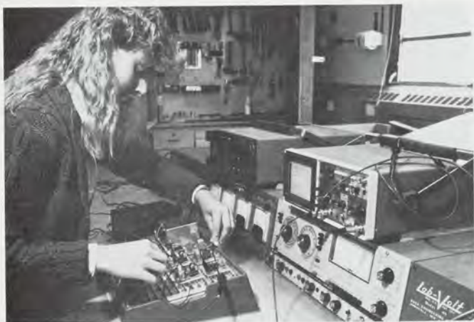
Senior Brenda Gold works with a dual-trace oscilloscope, used to detect problems in digital electronic equipment.
