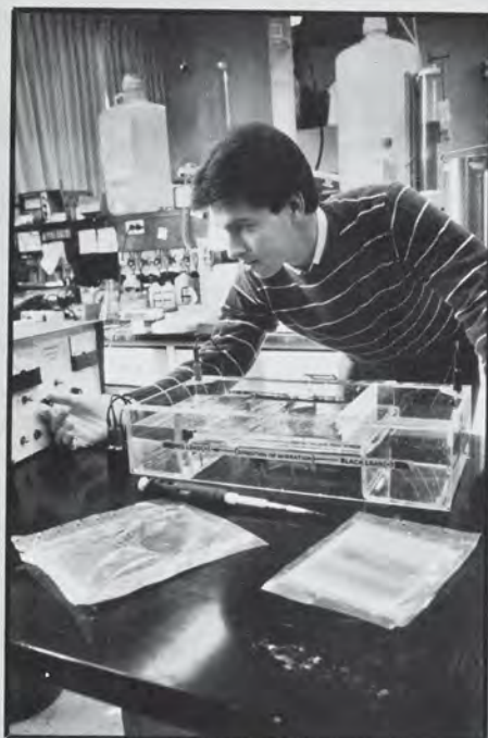
Jeff Johnson, doing research in biochemistry, adjusts the voltage on an electrophoresis apparatus.
