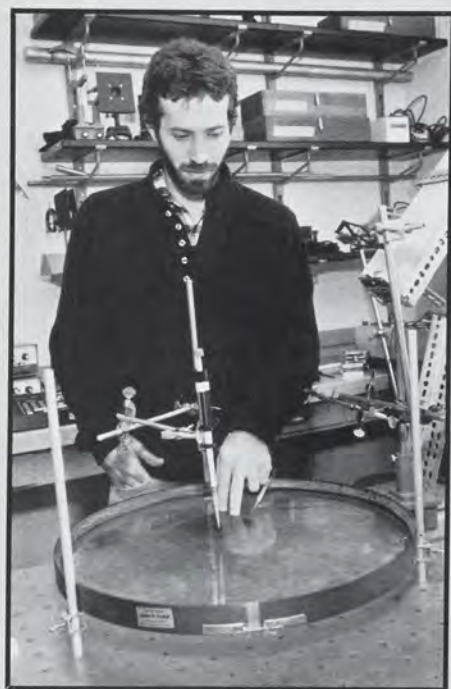
Using a water tank and a thin laser beam (invisible to the camera), Dan Winters can measure the velocity of a tiny wave.
