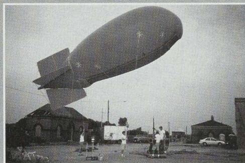
Students use a tethered balloon (about the size of a small car) to measure atmospheric ozone levels.
