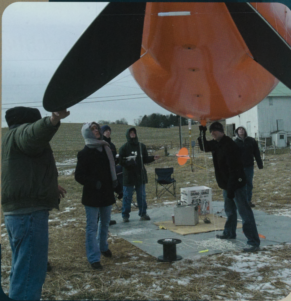
Tethered weather balloons (left) were used for collecting particles for a research study on winter air quality being conducted by Dr. Richard Clark (right).
