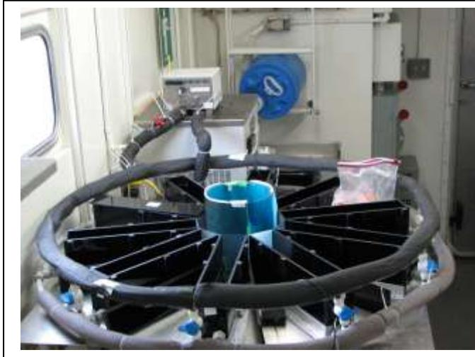
Figure 5. The radial photosynthetron, shown here in the radiation lab aboard the *Ron H. Brown*, measures the rate of CO<sub>2</sub> uptake in multiple samples from up to 10 depths simultaneously using a central light source. Ambient temperature (~ 5°
