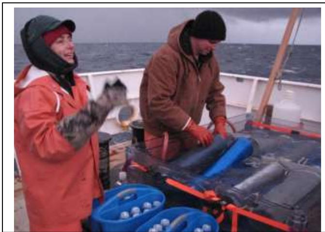
Figure 4. Scientists Dr. Veronica Lance (Lamont-Doherty Earth Observatory) and Dr. Pete Strutton (Oregon State University) arrange samples in on-deck incubator for 12-hour CO<sub>2</sub> uptake experiment on the back deck of the *Ron Brown*. The light source is natural sunlight, and temperature is maintained by flowing seawater pumped from the ship's side. The sample tubes are sheathed in blue filters to simulate the color of underwater light field.
