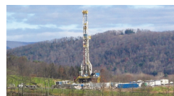
Tower for horizontal drilling into the Marcellus Shale in Lycoming County, Pennsylvania, USA. Photographer: Ruhrfisch (Wikimedia Commons)
