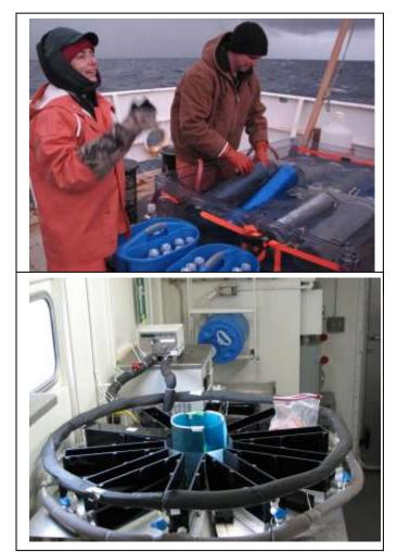
Figure 4. Scientists Dr. Veronica Lance (Lamont-Doherty Earth Observatory) and Dr. Pete Strutton (Oregon State University) arrange samples in on-deck incubator for 12-hour  $CO_2$  uptake experiment on the back deck of the *Ron Brown*. The light source is natural sunlight, and temperature is maintained by flowing seawater pumped from the ship's side. The sample tubes are sheathed in blue filters to simulate the color of underwater light field.
